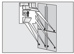
The number of lower brackets will depend on the width and design of the custom door.
